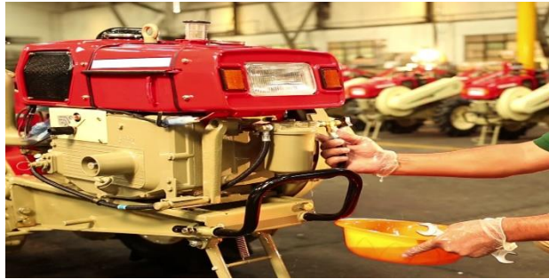
Fig. 3.10: Fuel filter in power tiller
