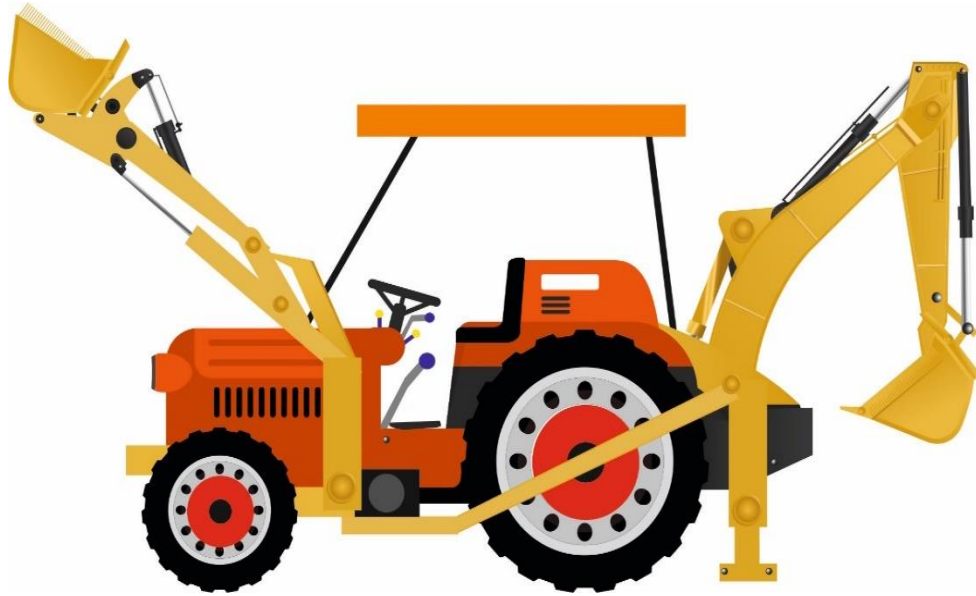
Fig. 2.7: Front end dozer and back hoe
